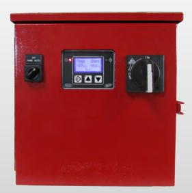
Metron's Model MP15 Jockey Pump is small, lightweight, technologically advanced microprocessor based controller intended for across-the-line starting of squirrel cage motors. MP15 controllers are for fire protection system applications where it is desirable to maintain uniform system water pressure by the use of an automatic pressure maintenance pump.
